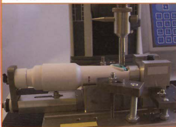
Figure 2: Assembly for testing the load required for button activation. The system is held in position using the custom-designed jig and force is applied to the actuation button.
